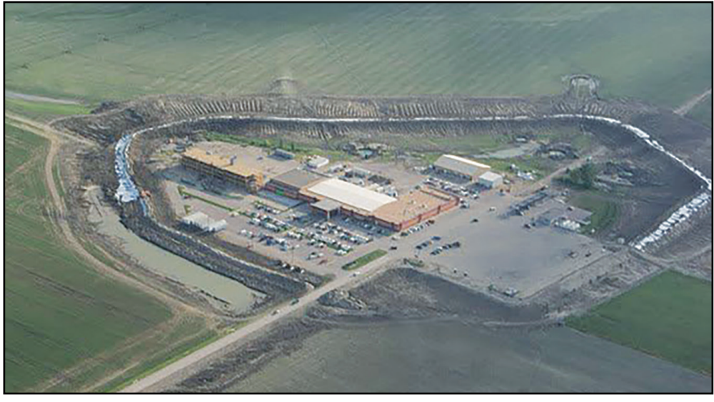
The flood of 2011 – here is an aerial shot of the berm put in place to prevent severe flooding at WinnaVegas Casino Resort. (Photo courtesy of Jerome LaPointe Sr.)
